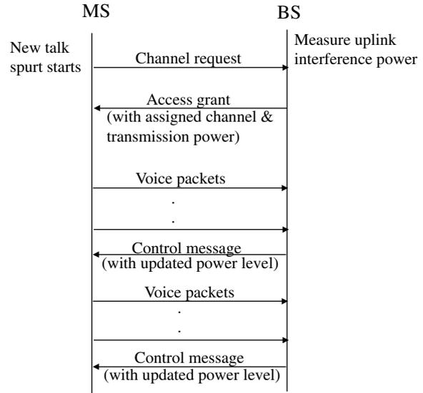
Fig. 2. Control messages for uplink transmission.
