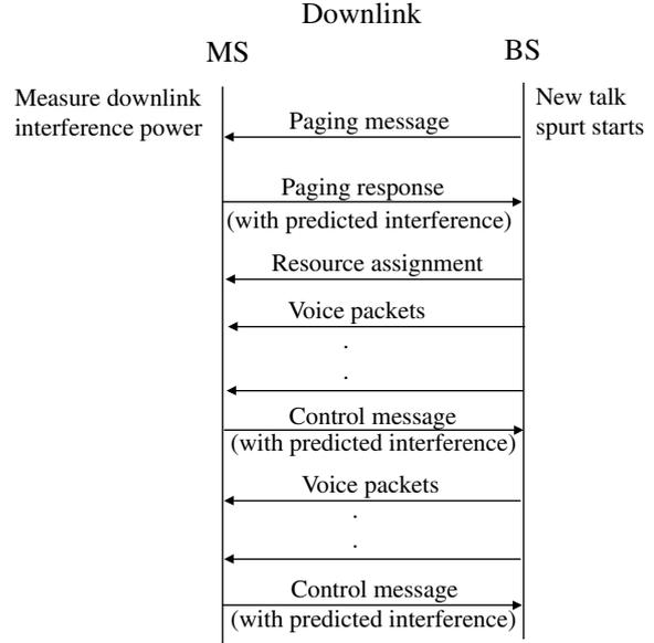
Fig. 1. Control messages for downlink transmission.
