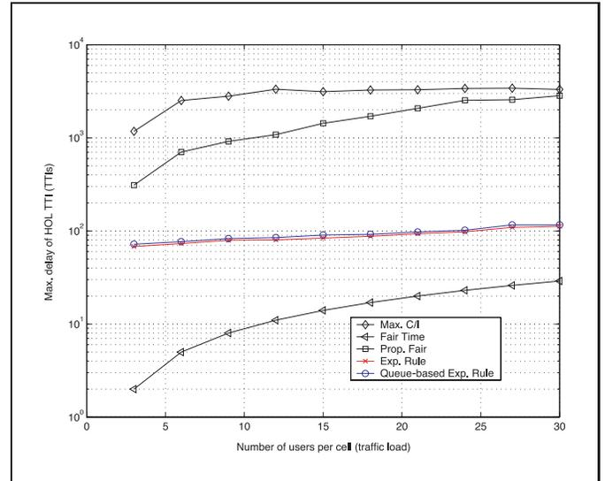
Figure 7: Maximum delay performance of all schedulers with multi-code operation in a time-multiplexing fashion.
