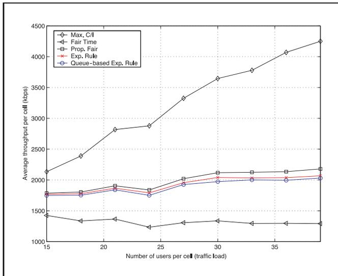
Figure 10: System throughput performance of all schedulers with multi-code operation in a code-multiplexing fashion.
