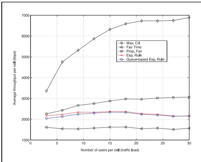
Figure 6: System throughput performance of all schedulers with multi-code operation in a time-multiplexing fashion.
