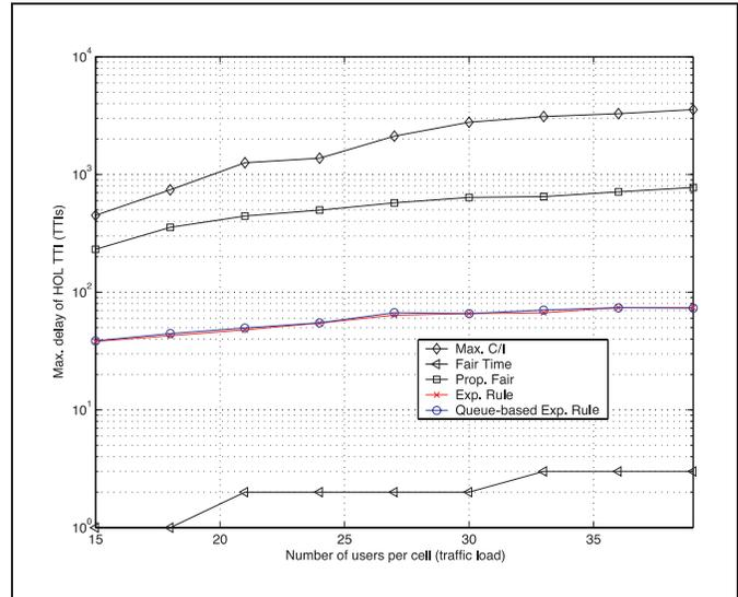
Figure 11: Maximum delay performance of all schedulers with multi-code operation in a code-multiplexing fashion.
