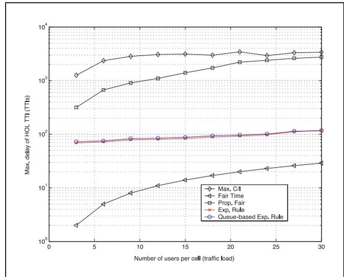
Figure 4: Maximum delay performance of all schedulers without multi-code operation in a time-multiplexing fashion.
