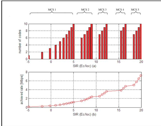
Figure 1: The hull curve with five modulation and coding schemes and the multi-code operation of maximum 10 codes [1].
