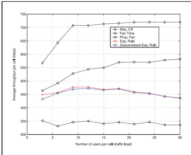
Figure 3: System throughput performance of all schedulers without multi-code operation in a time-multiplexing fashion.
