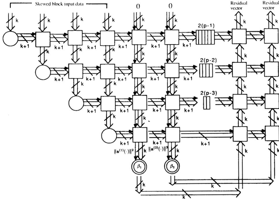
Fig. 7. MVDR beamforming using the SBHT systolic array.
