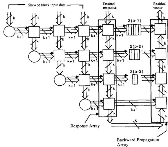
Fig. 4. New matrix-multiplication-free SBHT RLS systolic array.
