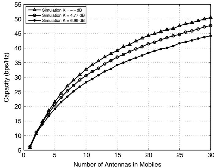
Fig. 9. The ergodic capacity of MIMO channels against the number of antennas when SNR = 20 dB,  $d = \lambda/2$  and  $I = N = 8$ .
