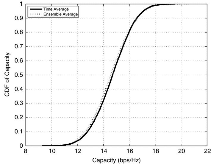
**Fig. 3.** The time and the ensemble average capacity CDF of a  $3 \times 3$  MIMO channel when  $K = 3$ , SNR = 20 dB, and  $d = \lambda/2$ .
