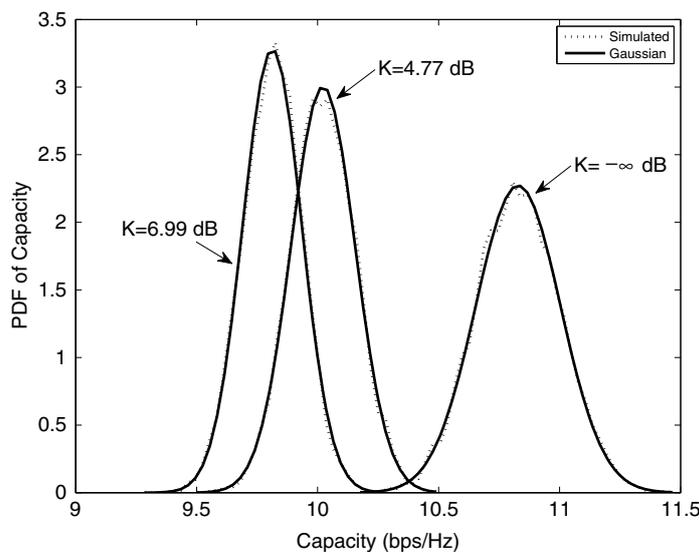
Fig. 5. Probability density functions of MIMO capacity in a mobile-to-mobile Rician fading channel.
