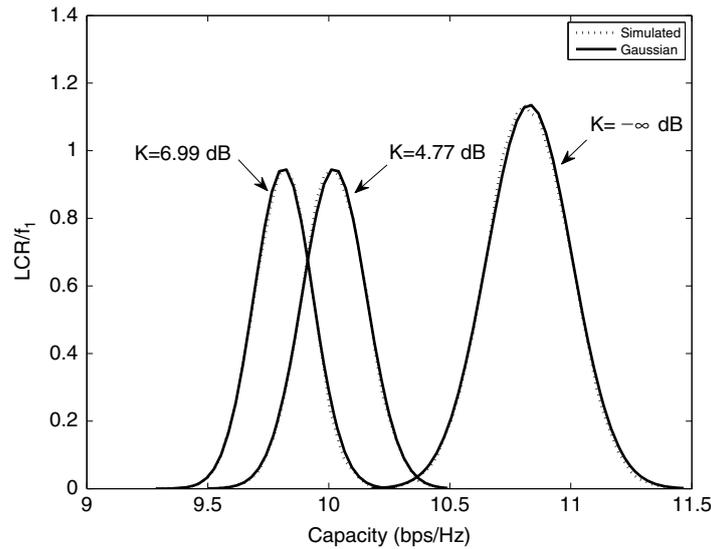
Fig. 6. Level crossing rate of the MIMO capacity in a mobile-to-mobile Rician fading channel.  $f_1$  is the maximum Doppler frequency of the transmitter.
