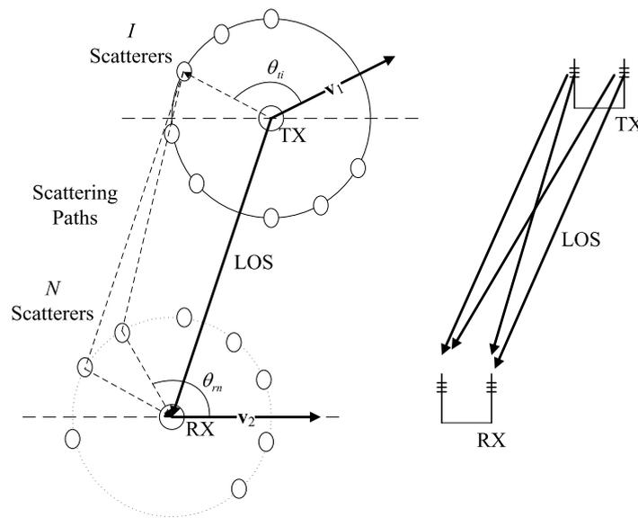
Fig. 1. Double-ring scattering model with LOS components.
