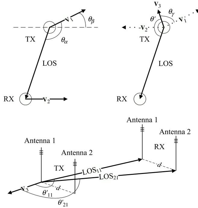
**Fig. 2.** LOS component model for moving transmitter TX and receiver RX of which velocity vectors are  $\mathbf{v}_1$  and  $\mathbf{v}_2$  with a relative angle of  $\theta_\beta$ , respectively.
