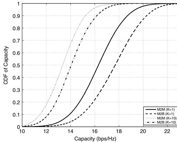
Fig. 4. The CDF of capacity of mobile-to-mobile (M2M) and mobile-to-base-station (M2B) channels for Rician factor  $K = 1$  and  $10$ .
