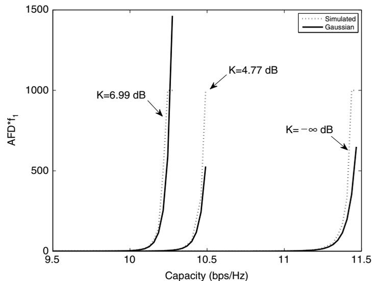
Fig. 7. Average fading duration of the MIMO capacity in a mobile-to-mobile Rician fading channel.  $f_1$  is the maximum Doppler frequency of the transmitter.
