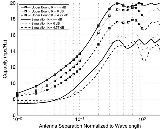
Fig. 8. Effect of antenna separation on the ergodic capacity of a  $3 \times 3$  MIMO channel for SNR = 20 dB and various values of  $K$  factors.
