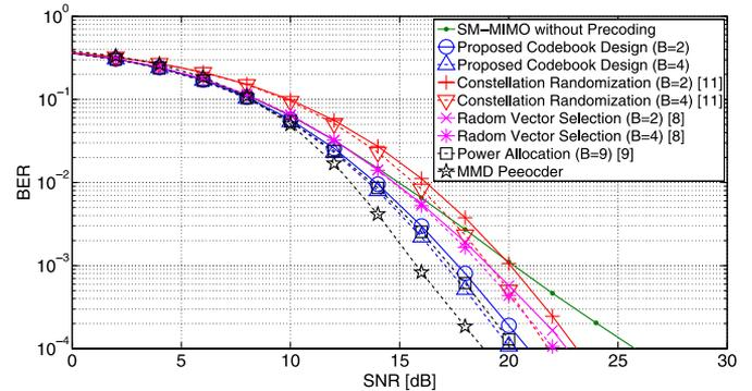
Fig. 3. BER evaluation of different designs for SM-MIMO systems with  $N_t = 8$ ,  $N_r = 2$ , and  $M = 4$  (QPSK) in uncorrelated Rayleigh fading channels.
