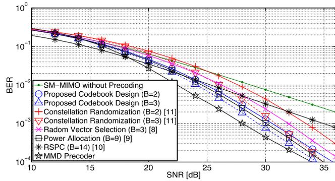
Fig. 2. BER evaluation of different designs for SM-MIMO systems with  $N_t = 8$ ,  $N_r = 1$ , and  $M = 4$  (QPSK) in uncorrelated Rayleigh fading channels.
