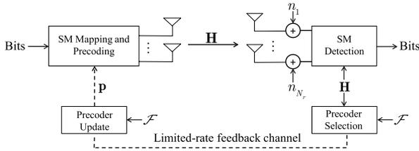
Fig. 1. System model for SM-MIMO with limited feedback precoding.
